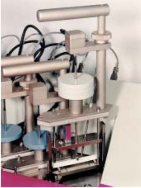
HDT test station
